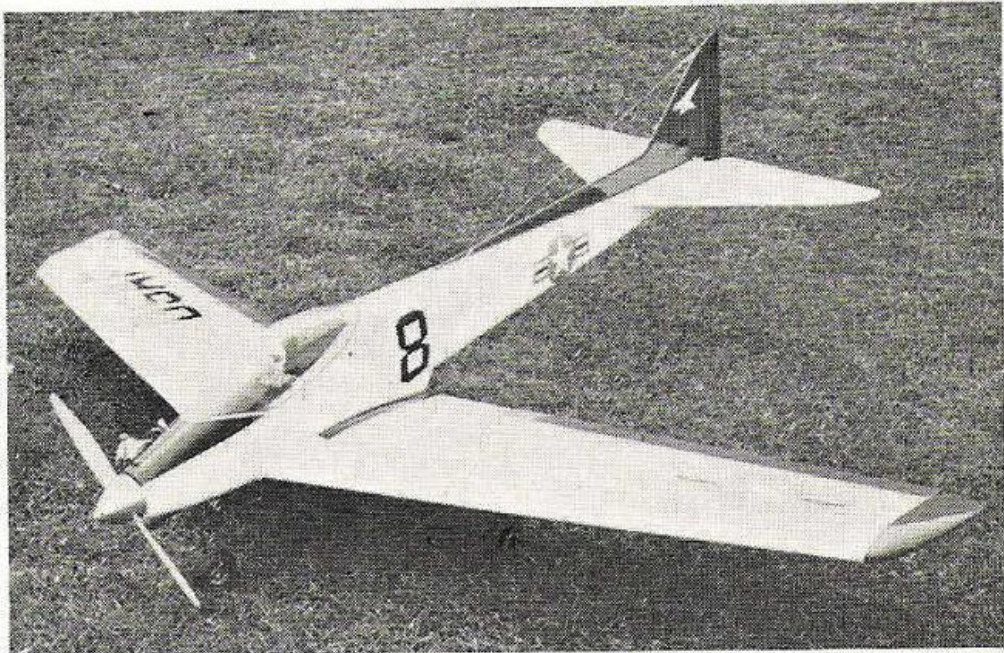
These views of Mike Young's "CHEVRON" show the fighter-ish lines of this racy looking model. Note side-mounted engine.
