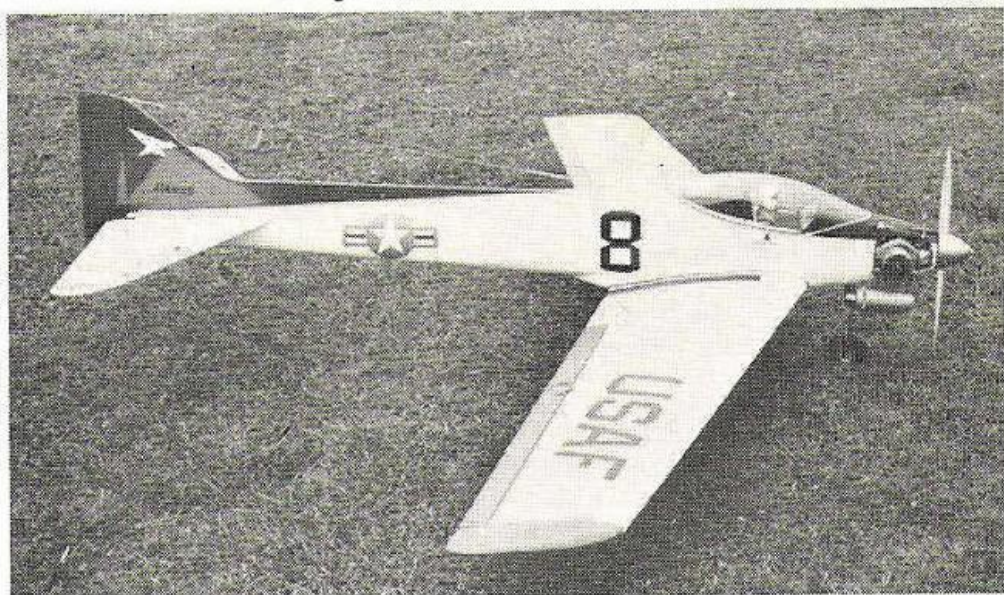
These views of Mike Young's "CHEVRON" show the fighter-ish lines of this racy looking model. Note side-mounted engine.
